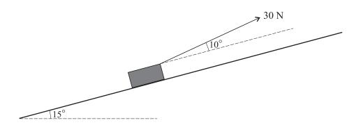
A box of mass 8 kg is pulled, at constant speed, up a straight path which is inclined at an angle of  $15^{\circ}$  to the horizontal. The pulling force is constant, of magnitude 30 N, and acts upwards at an angle of  $10^{\circ}$  from the path (see diagram). The box passes through the points *A* and *B*, where AB = 20 m and *B* is above the level of *A*. For the motion from *A* to *B*, find
