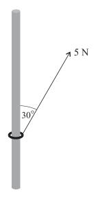
A small ring of mass 0.6 kg is threaded on a rough rod which is fixed vertically. The ring is in equilibrium, acted on by a force of magnitude 5 N pulling upwards at  $30^{\circ}$  to the vertical (see diagram).
